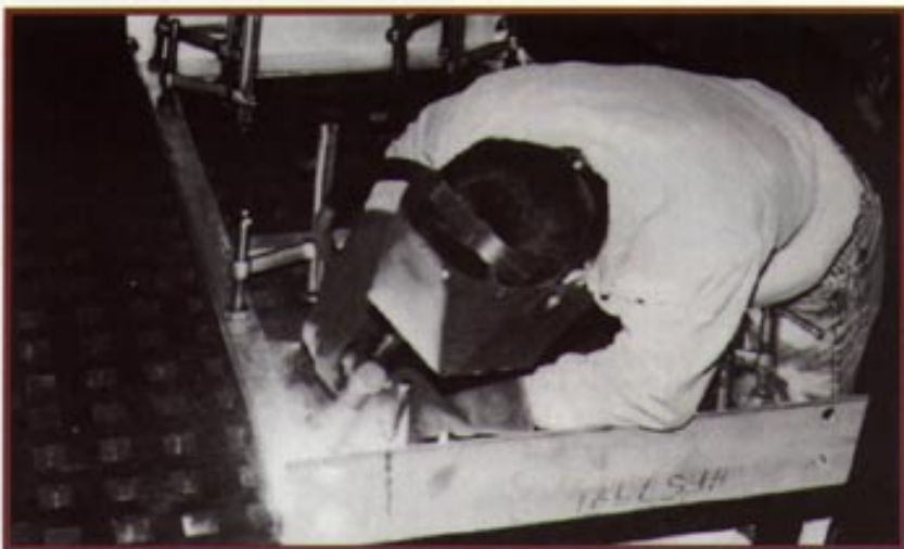
Figure 3 Vertical slide clamps are used on a platen.
